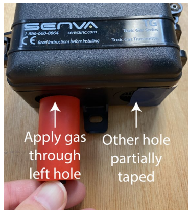
Figure 3: Applying test gas with enclosure closed.
